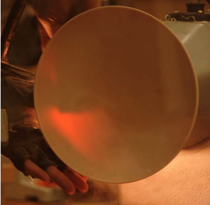
The lamp is aimed at the outside of the bowl and as the bowl is turned and hollowed out light from the lamp shines through the side of the bowl aiding in getting a uniform thin wall
