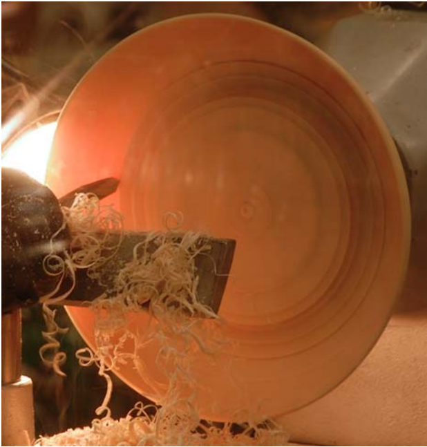
Once a section has been thinned, do not go back and try to thin it some more since the thin wall will be flexing and possibly warping.
