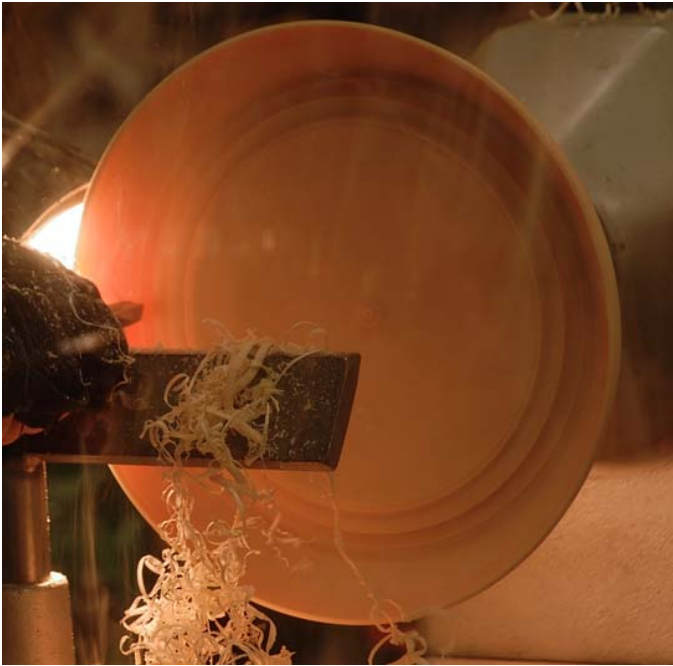
The lamp is aimed at the outside of the bowl and as the bowl is turned and hollowed out light from the lamp shines through the side of the bowl aiding in getting a uniform thin wall
